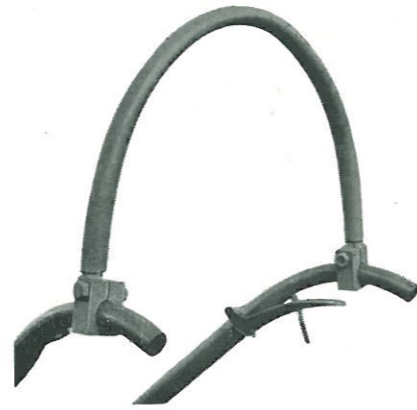
A special handlebar extension can be quickly fitted.
