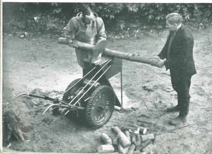
Logs up to 6-in. in diameter can be cut in one passage
