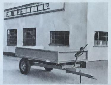
The robust 'Anglia' Trailer of  $3/3\frac{1}{2}$  ton capacity incorporates the usual high quality 'Pettit' design and finish at low cost.
