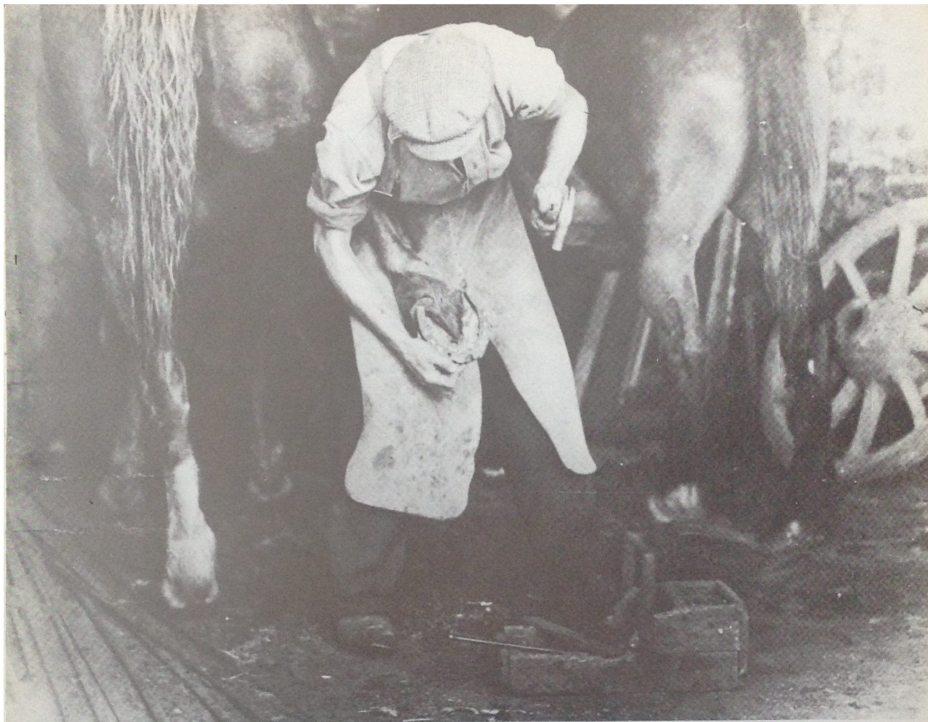
ABOVE: Fitting the shoe – the final stage of nailing the shoe on to the hoof. COVER: A page from the Samuel Lewis catalogue, c. 1920.
