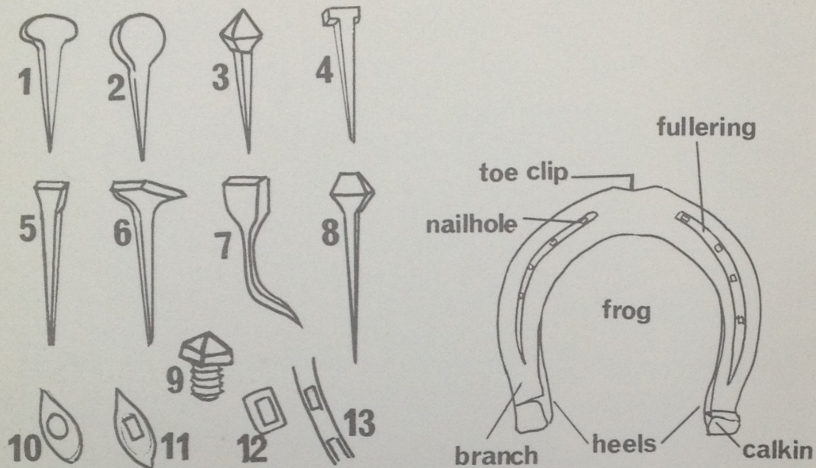
LEFT: Types of nails and nail-holes used in securing horse, ox and mule-shoes. 1. Fiddle-headed nail; 2. Round-headed nail; 3. Spiked nail (also known as frost nail); 4. T-headed nail; 5. Square-headed nail; 6. Ox-shoe nail; 7. Mule nail; 8. French horse nail; 9. Screw-in frost stud or calk; 10. Early round hole in punched oval countersunk shoulder; 11. Norman square hole in punched oval countersunk shoulder; 12. Square-punched hole and recessed; 13. Square hole in fullered groove. RIGHT: Main parts of the horseshoe.
