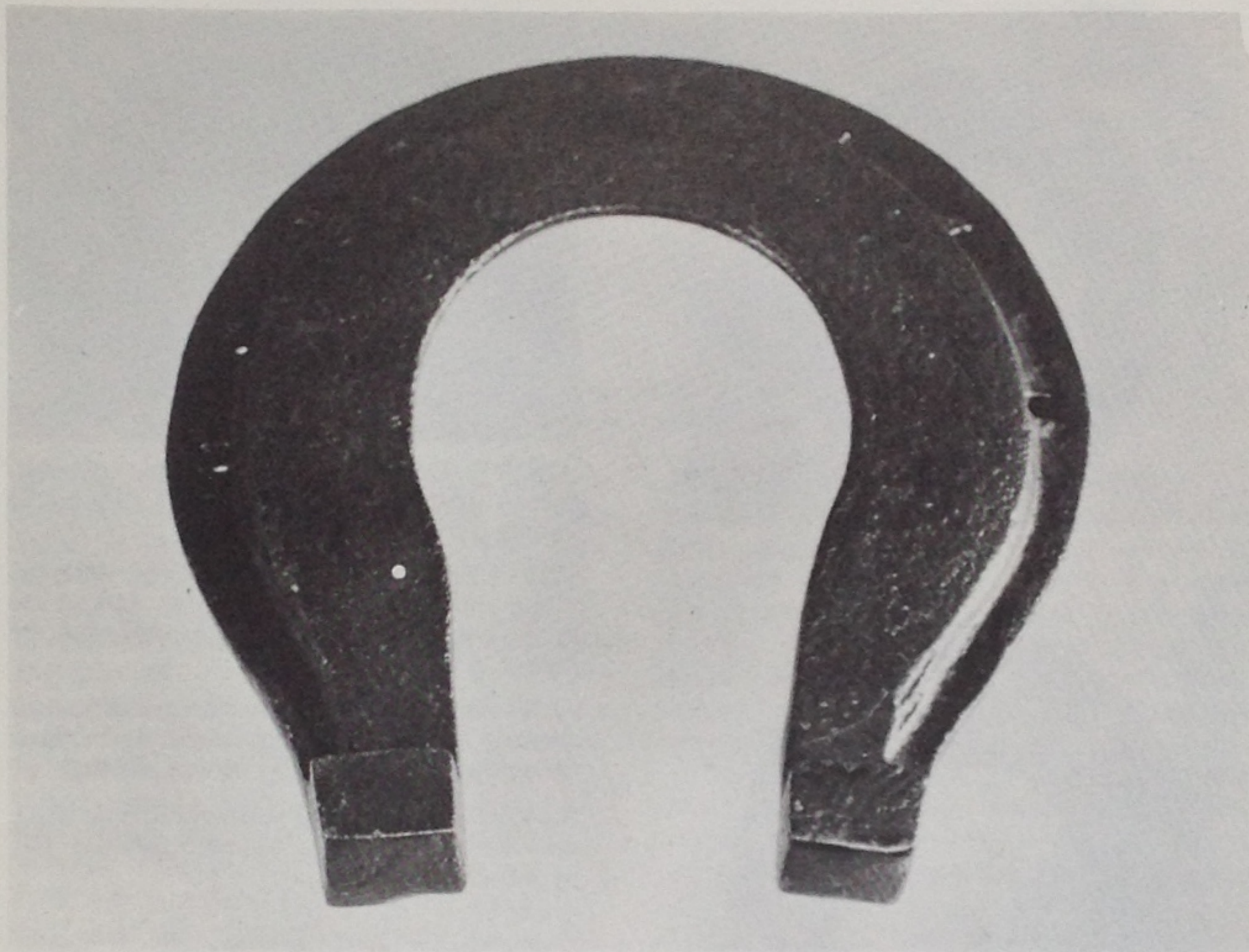
Beautiful example of a very late keyhole shoe with rim-fullered groove and heavy calkins, possibly early nineteenth century.
